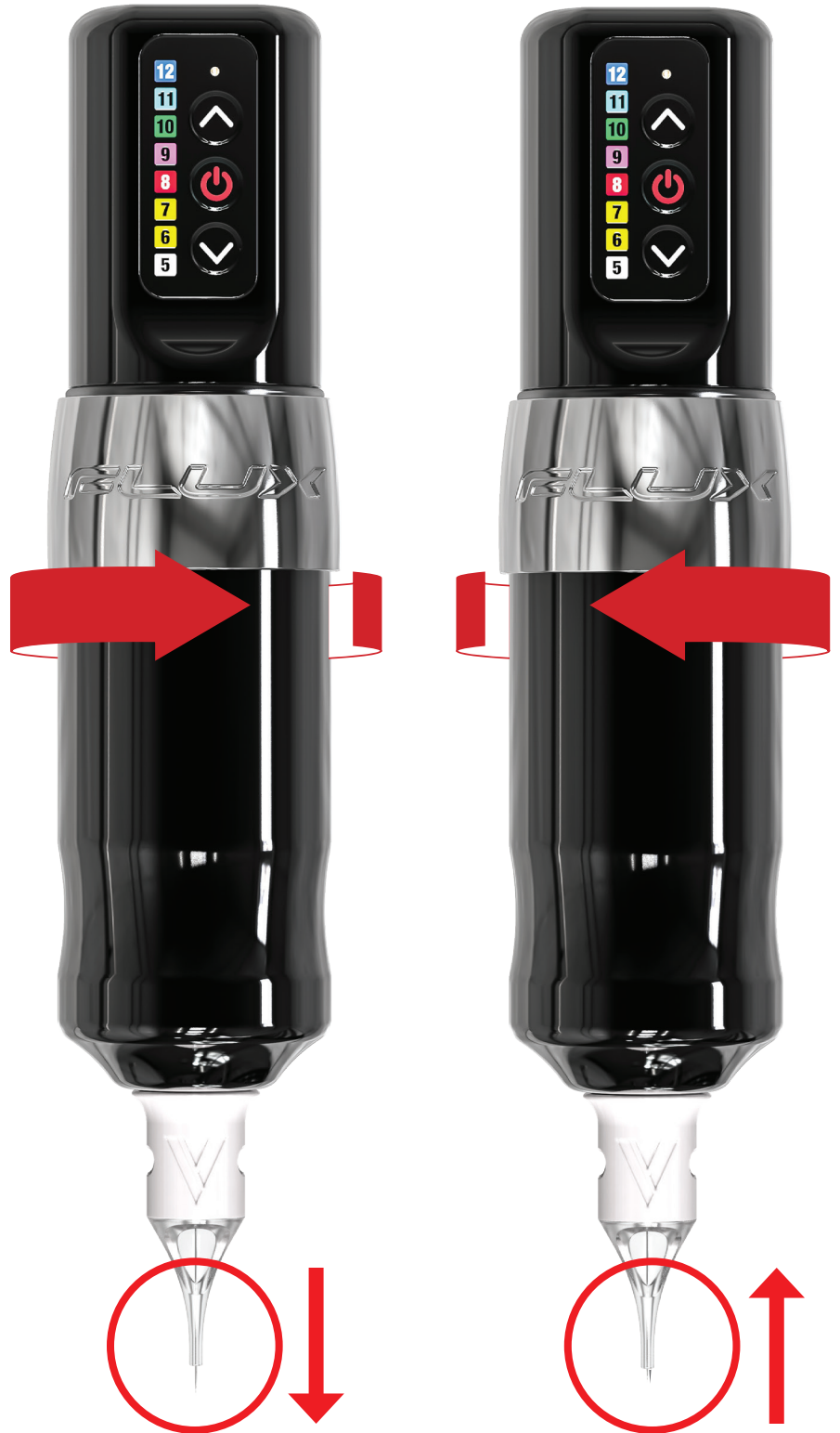
Turning the grip as shown increases needle depth.
